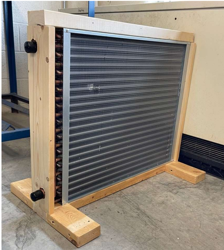
Figure 35: Wooden frame built for the Heat Exchanger
